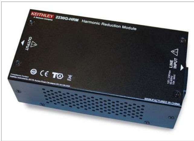
2230G-HRM Harmonic Reduction Module reduces AC power line current harmonics when inserted between the power supply and the power outlet. The 2230G-HRM is required for compliance to standard EN 61000-3-2 in EU countries and is needed for the 2230-30-6 and 2230-60-3.
