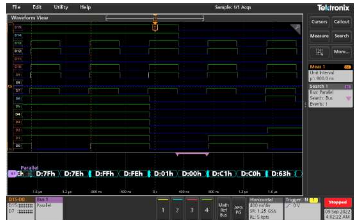
Digital channel trigger and decode
