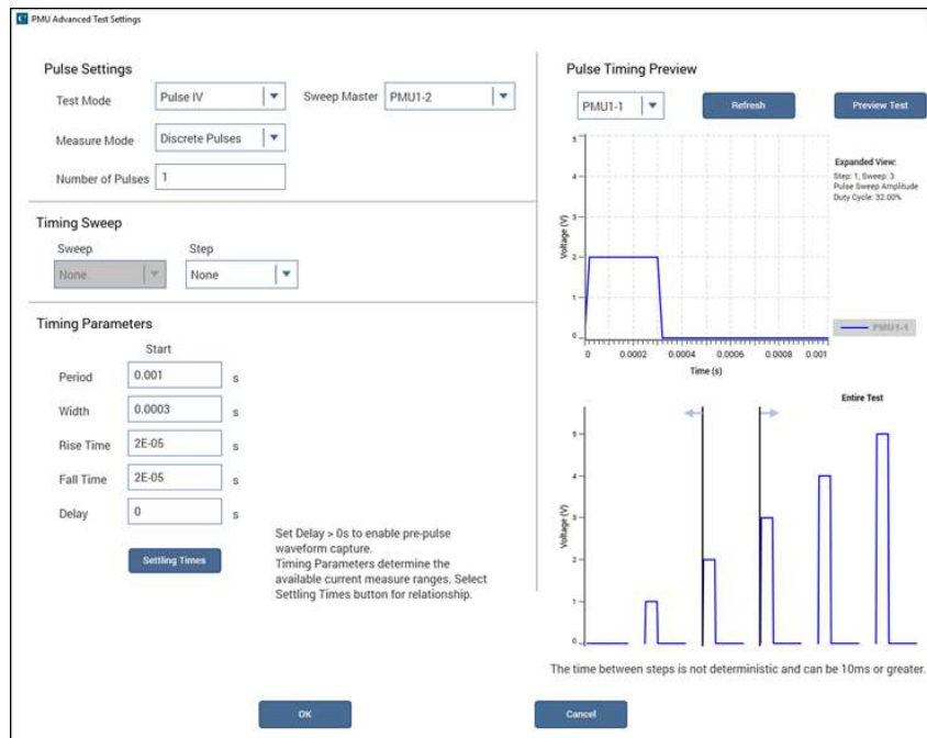
Figure 57: Six-point pulse amplitude sweep
