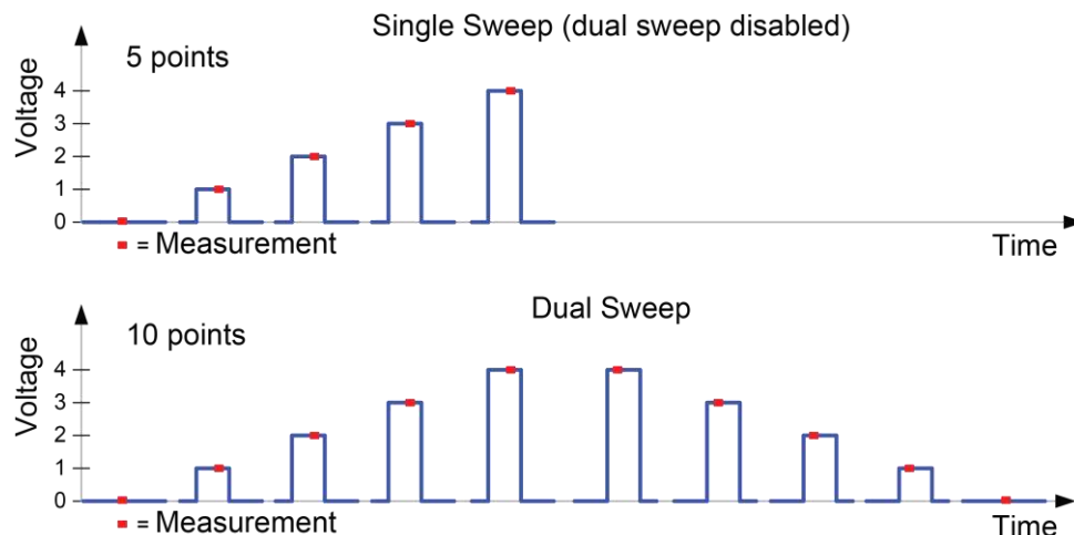
Figure 35: Single and dual pulse amplitude sweep examples
