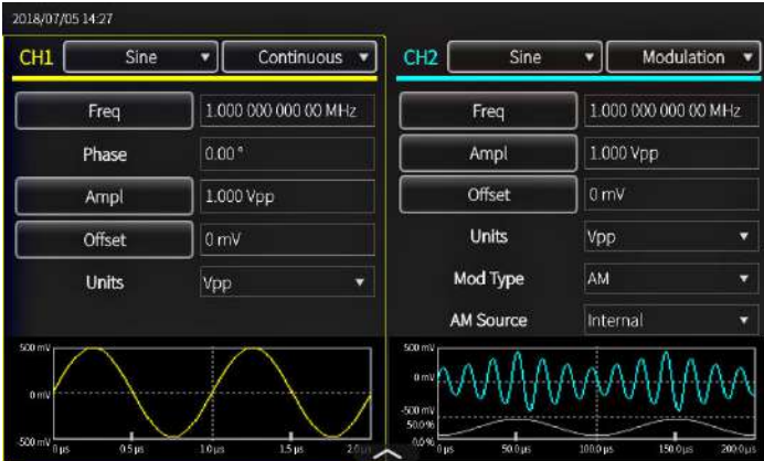
Key settings are visible at a glance, and are easy to adjust using touch, numeric keypad, or rotary controls
