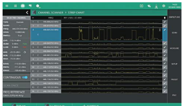
The Strip Chart Mode Tracks Signal Level of All Channels Over Time.
