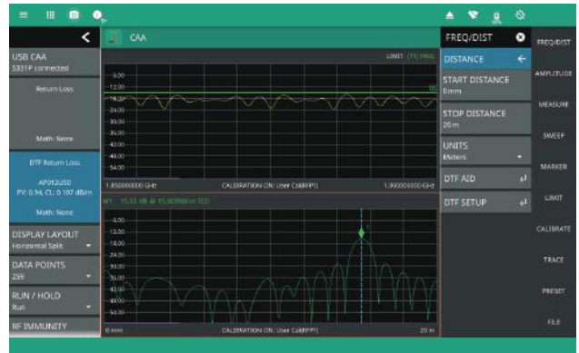
Simultaneous Display of Cable and Antenna Feed Return Loss and Distance to Fault
