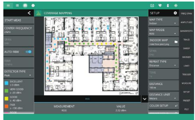
Typical Result Screen for Indoor Coverage Mapping
