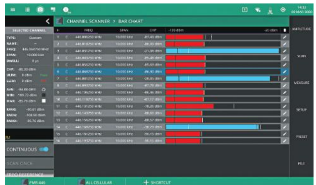
The Bar Chart Displays the Current Signal Level of Up to 20 Channels on a Single Screen
