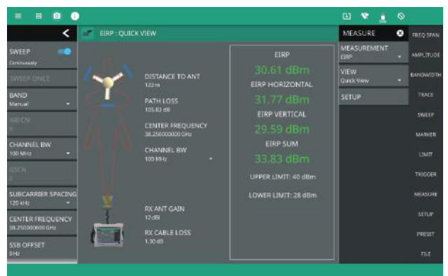
The EIRP Results "Quick View" Screen Provides a Graphical Display of Measurement Configuration and Total EIRP Power
