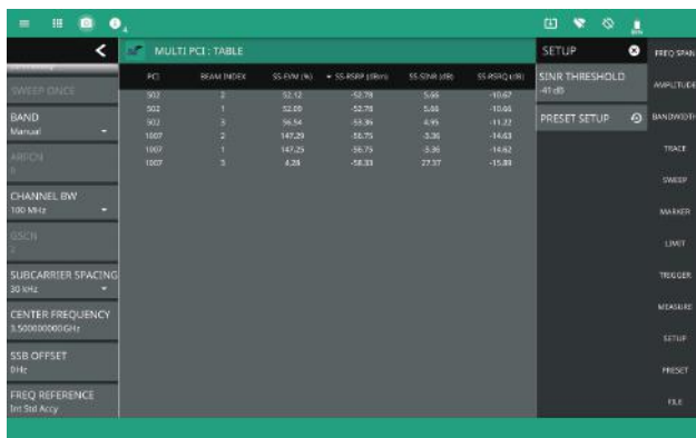
Field Master Pro MS2090A Offers Multi-PCI Measurements for OTA Testing of One or More 5G NR gNB
