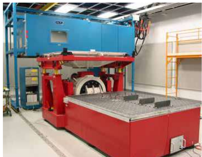
AGREE Temperature, Humidity Chamber interfaced with Vibration Shaker Table
