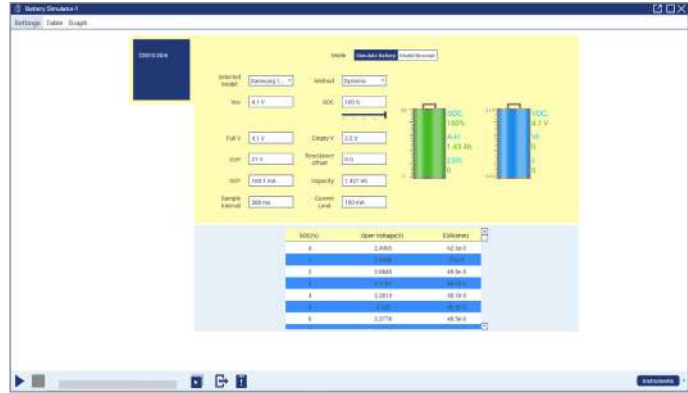
The Battery Simulator App allows users to simulate battery models and monitor key parameters in real time.
