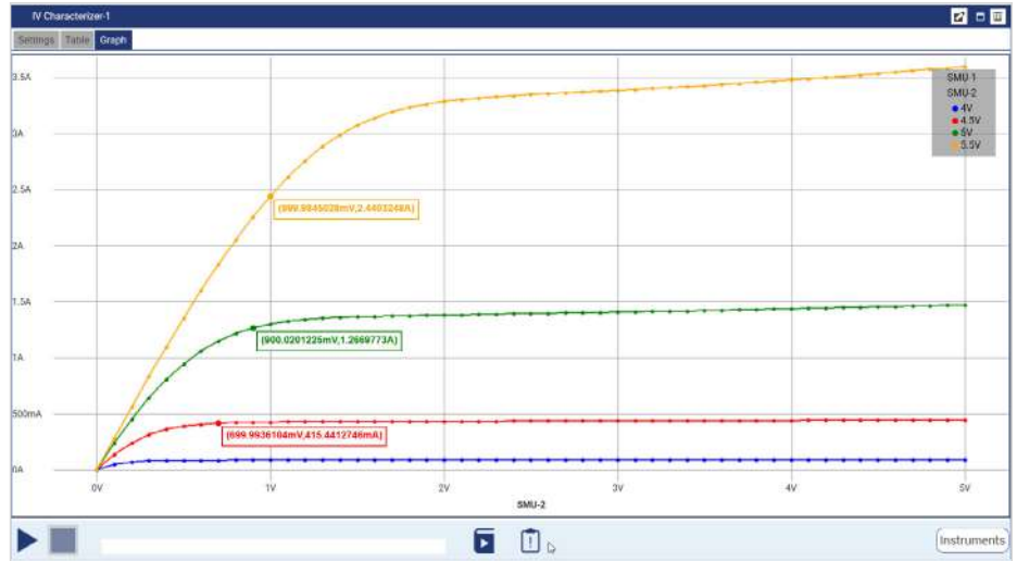
Create current vs. voltage characteristics for 2-terminal, 3-terminal, and 4-terminal devices.
