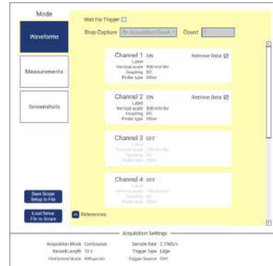
The setup window enables the selection of the Waveforms, Measurements, or Screenshots mode.
