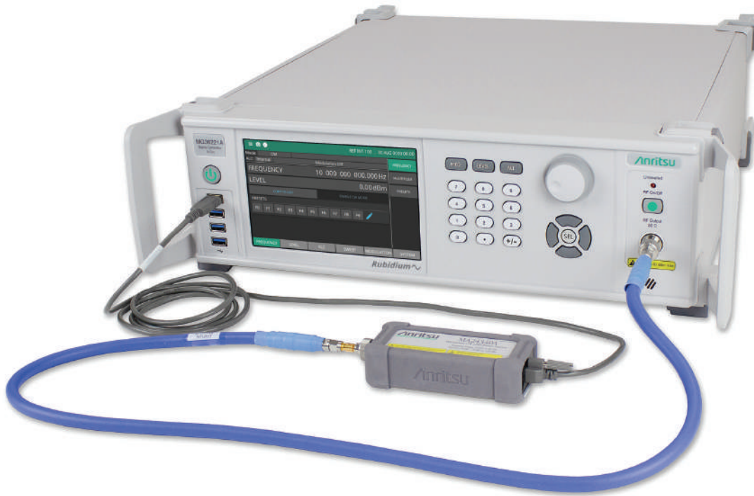
Rubidium MG362x1A Signal Generator Connected to a MA243xxA Power Sensor
