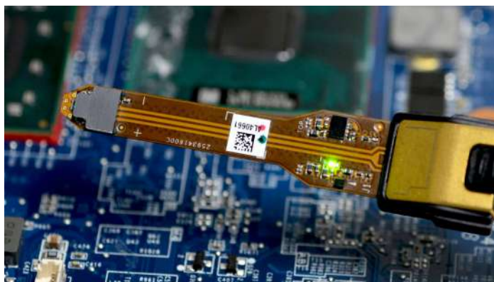
P77STFLXA solder down, flex-circuit accessory with an active buffer amplifier on its tip.
