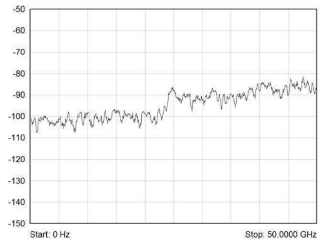
Typical Isolation (dB) Plot for 50 GHz Terminated & Unterminated Versions
