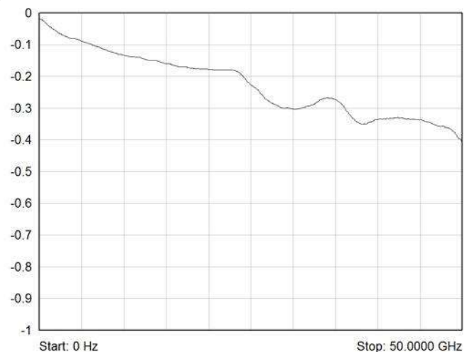
Typical Insertion Loss (dB) Plot for 50 GHz Terminated & Unterminated Versions
