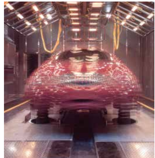
Four post road simulator with temperature, humidity, vibration and solar simulation.
