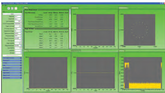
GSM/EDGE Uplink TX Measurement using CombiView
