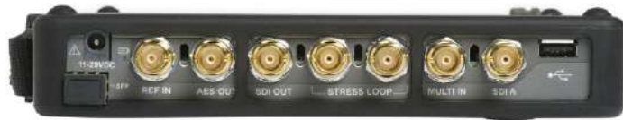
WFM2200A top panel connectors.
