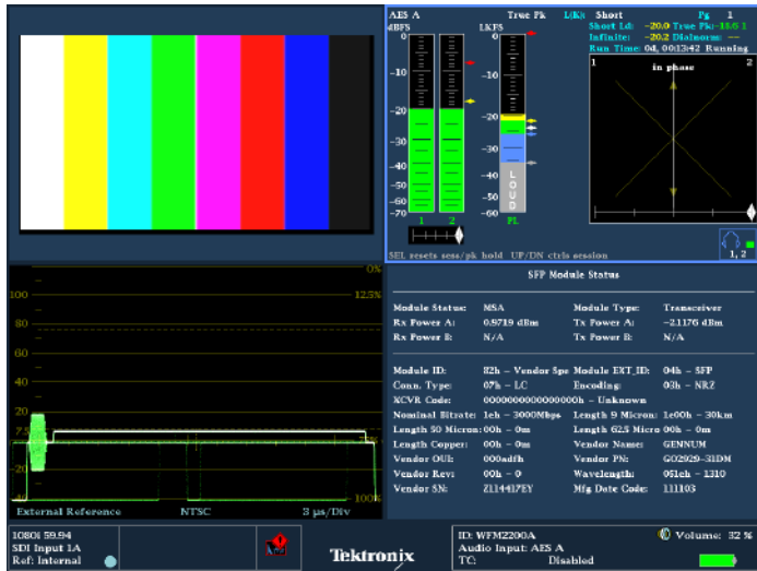
Variety of interface support (Picture display, Audio Phase display of AES/EBU input with Loudness Meter, Waveform display of external reference input, SFP Module Status display of optical input).
