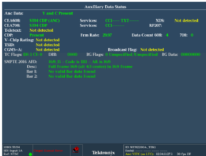
Monitoring of Ancillary data (Closed Caption, Time Code, and AFD) using Aux Data Status.
