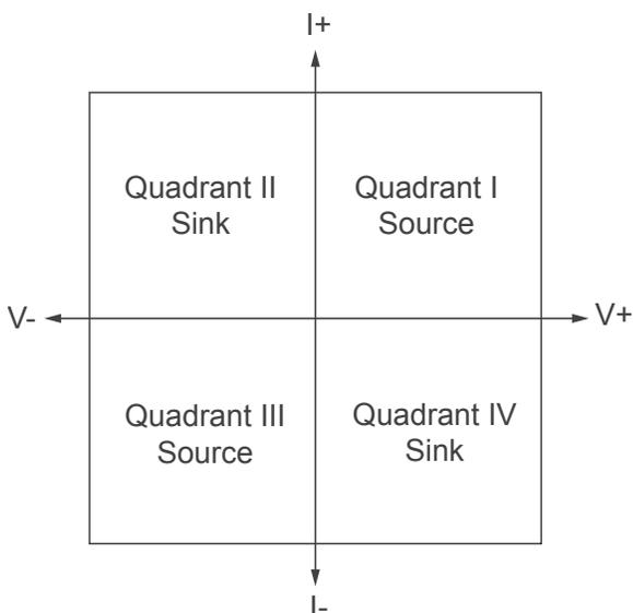
For example, when you have a positive voltage and current flowing out of the positive terminal (that is, a positive current), the output operation falls within Quadrant I and is sourcing power. When you have a positive voltage and a current flowing into the positive terminal (that is, a negative current), the output operation falls within Quadrant IV, and is sinking power.
