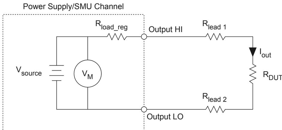
When the PXIe-4137 is operating in Constant Voltage mode, local sense forces the requested voltage at the output terminals of the module. The actual voltage at the DUT terminals is lower than the requested output because of the output lead resistance error.
