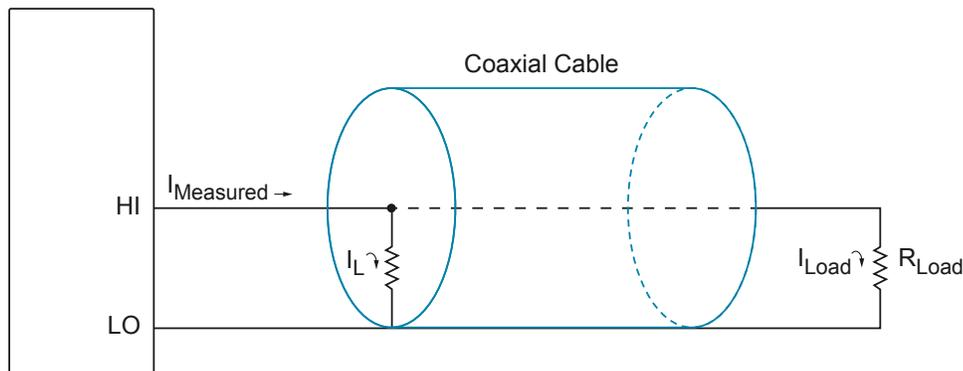
**Figure 14.** Reducing Leakage with Guarding ( $I_{\text{Measured}} = I_{\text{Load}}$ )
