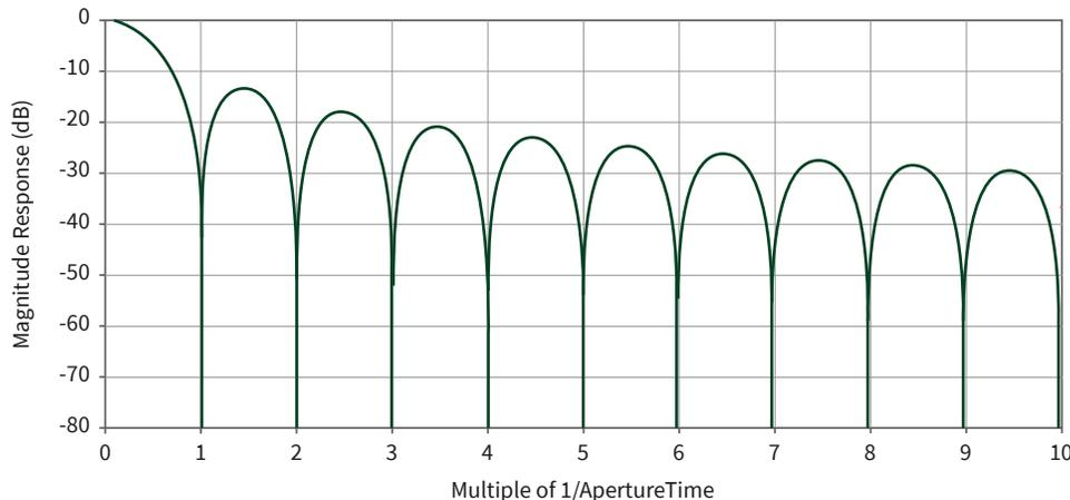
The best frequency rejection is available only near integer multiples of  $1 / \text{Aperture Time}$ . You can achieve the fastest possible readings along with good power-line noise rejection by setting the aperture to one power-line cycle (PLC) and noise rejection to Normal.
