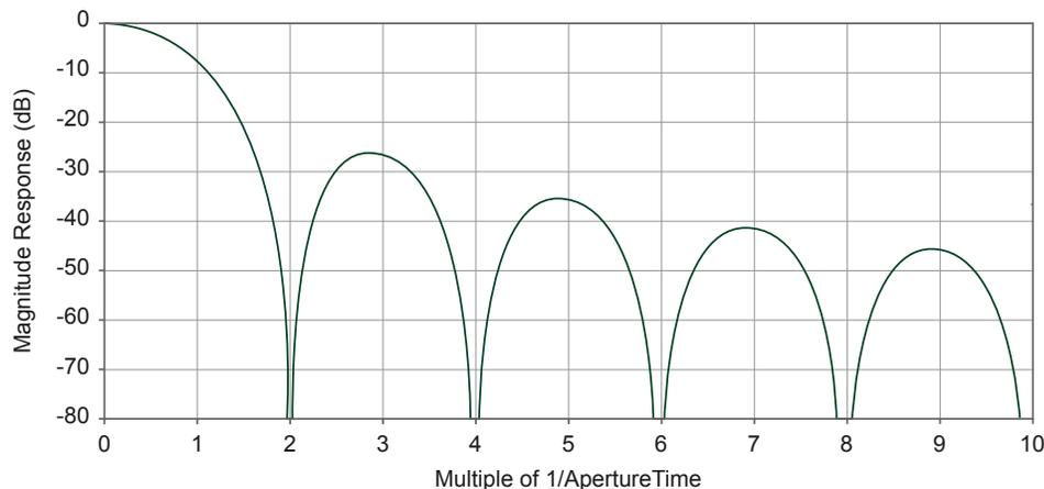
With second-order noise rejection, the instrument provides superior noise rejection even near multiples of  $1 / \text{Aperture Time}$ , and noise rejection increases more rapidly with frequency compared to normal noise rejection. Notches are also wider than they would be with normal weighting, which results in less sensitivity to slight variations in noise frequency.
