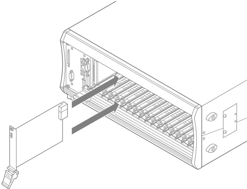
9. Place the module edges into the module guides at the top and bottom of the chassis. Slide the module into the slot until it is fully inserted.
