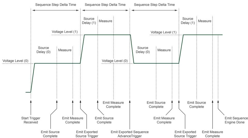
When an NI-DCPower instrument uses sequence step delta time, the source unit operates according to the following steps:
