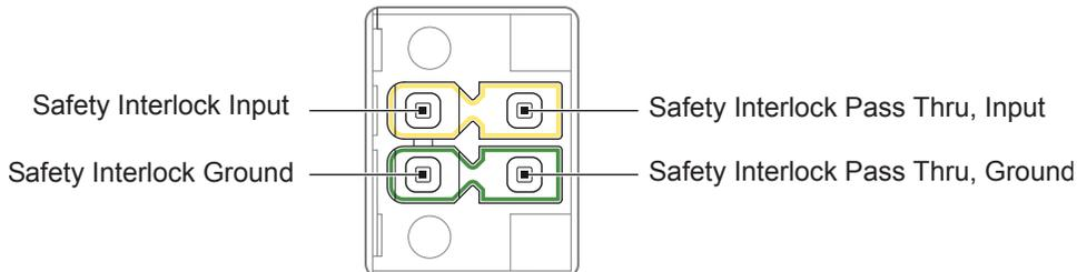
Complete the following steps to connect the safety interlock subsystem with generic cabling.
