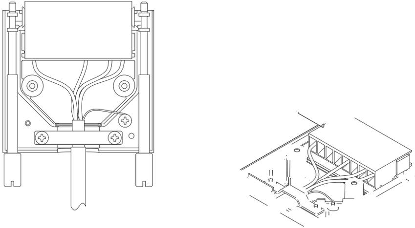
1. Strain relief clamped onto ground shield
